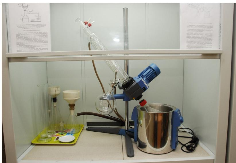
**Figure 3.** Photo of evaporator
